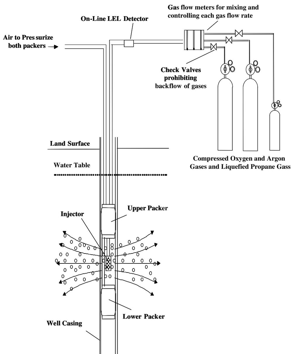
Fig. 1. Experimental set-up for direct gas-sparging into the saturated aquifer.
