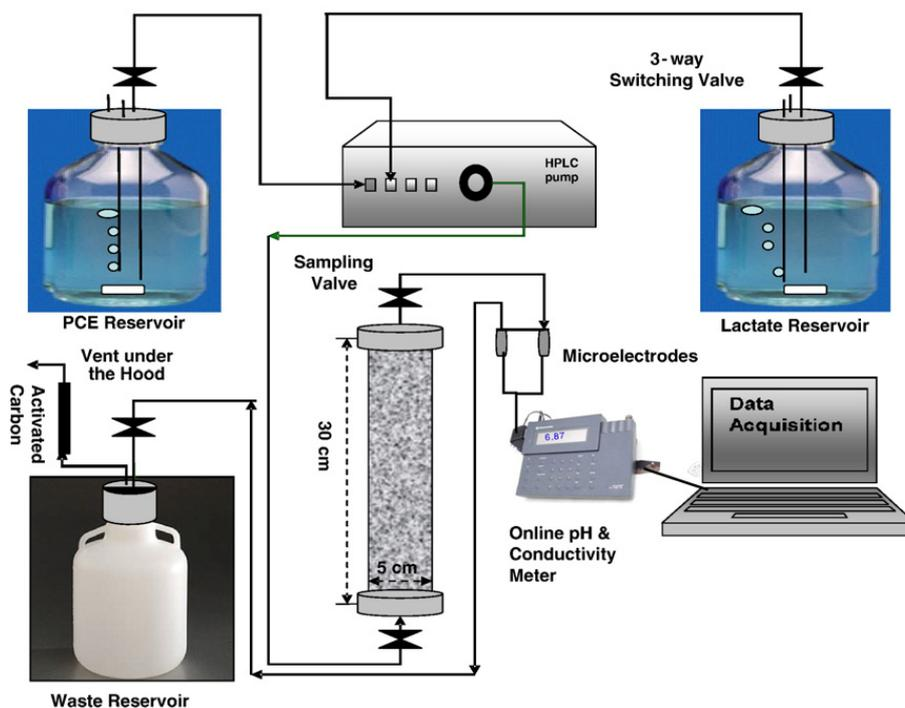
Fig. 1. Schematic of experimental setup and column design. The column was made from pyrex and connected with PEEK tubing.
