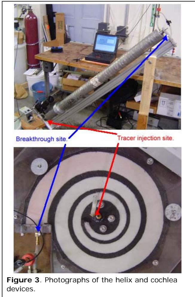
The helix and cochlea methods are appealing for their simplicity. They allow accurate measurement of the illusive property of transverse dispersion with a procedure similar to a classic column experiment.
